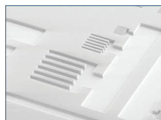
AR-P 6510.17 Film thickness 40 µm, structures up to 5 µm (synchrotron)
