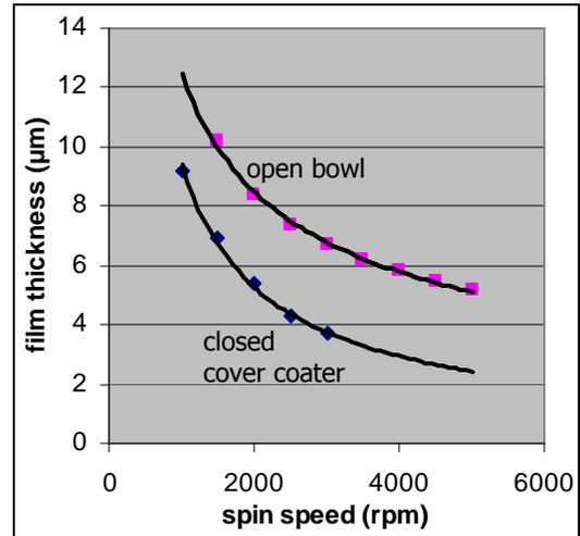
**Figure 3.** Spin curves of CYCLOTENE 4024-40 resin in open and closed bowl configurations. Spin time was 30 seconds.
